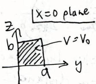
$$\nabla^2 V = 0 \Rightarrow \frac{\partial^2 V}{\partial x^2} + \frac{\partial^2 V}{\partial y^2} + \frac{\partial^2 V}{\partial z^2} = 0$$
